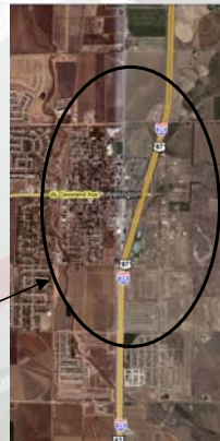
Slight curves in the highway alignment at Wellington, CO impose 130-mph speed restriction
