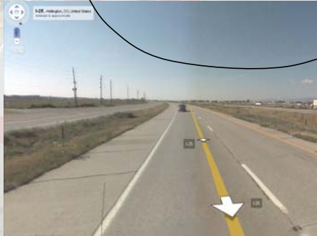
Slight curves in the highway alignment at Wellington, CO impose 130-mph speed restriction
